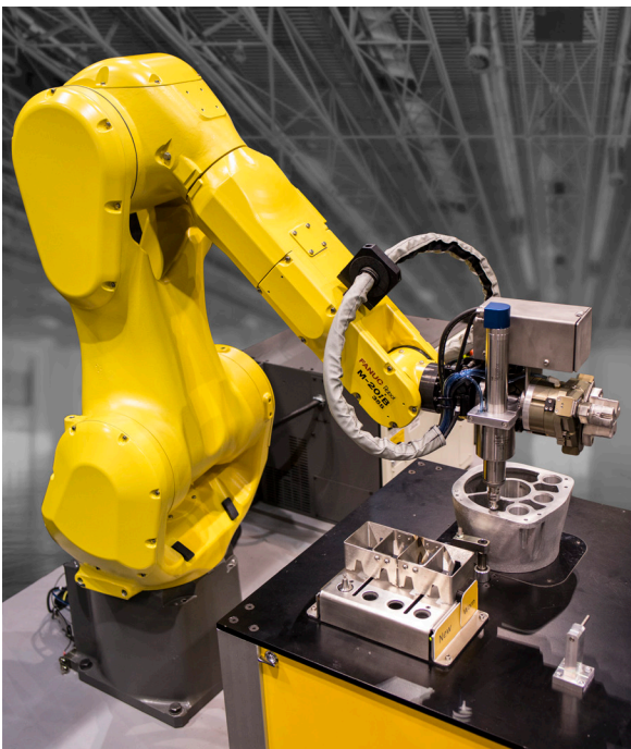
M-20 i B/35S deburring casted parts
