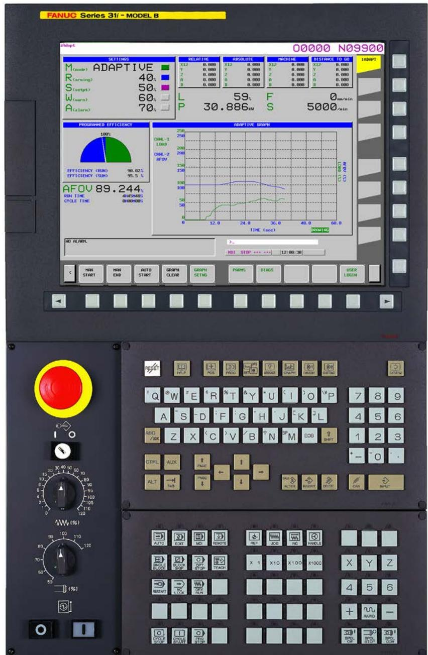
Figure 17. Adaptive control during roughing complements high-speed machining during finishing.
