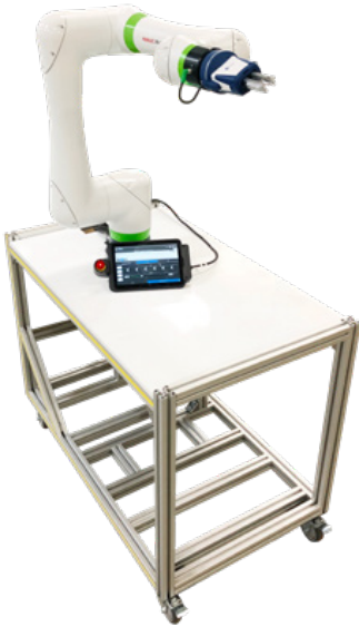
STANDARD CART: Aluminum structure with steel table
