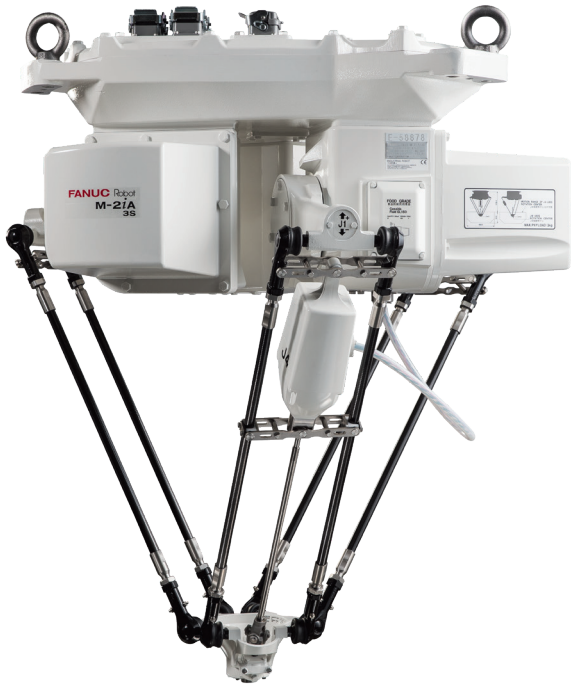
M-2iA/3S 4-axis, hollow rotational wrist
